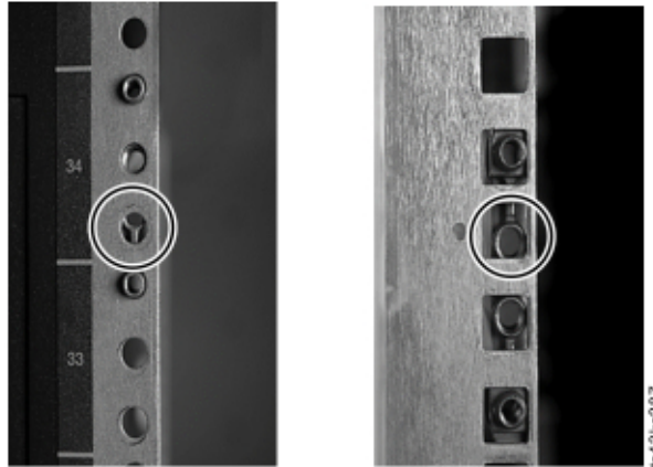
Figure 36. Incorrect connector locations
