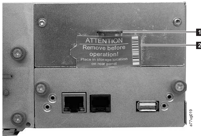
Figure 181. Library shipping lock and label storage location on the rear panel of the library
