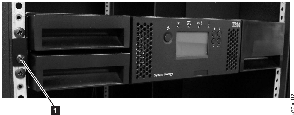
Figure 178. Removing the two mounting bracket screws anchoring the library to the rack (one screw on each side of the library)
