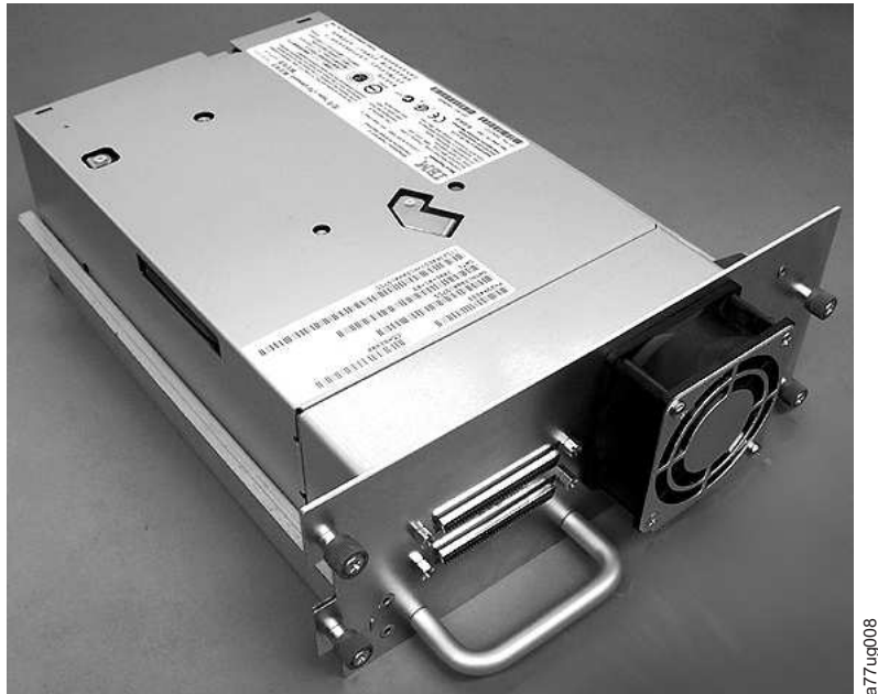
Figure 167. Library drive sled without ElectroStatic Discharge (ESD) springs (SCSI sled shown)
