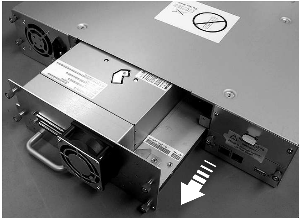
Figure 170. Pulling the drive sled out of the library (drive sled without ESD springs shown)
