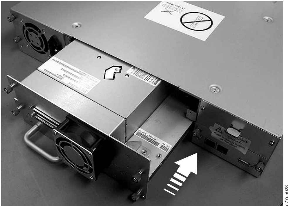
Figure 171. Pushing the drive sled into the library (drive sled without ESD springs shown)
