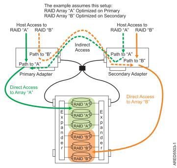
Figure 26. Dual storage IOA optimization. This figure shows RAID arrays with primary and secondary adapters.
