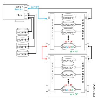
Figure 44. Example of SAS subsystem unit addresses
