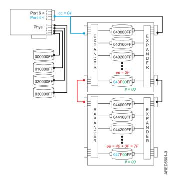
Figure 43. Example of SAS subsystem unit addresses
