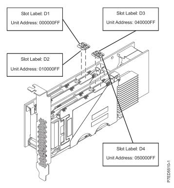
Figure 10. CCIN 57CD PCIe SAS RAID and SSD adapter 3 Gb x8
