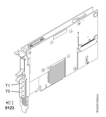
Figure 9. CCIN 574E PCIe x8 Ext Dual-x4 3 Gb SAS RAID adapter
