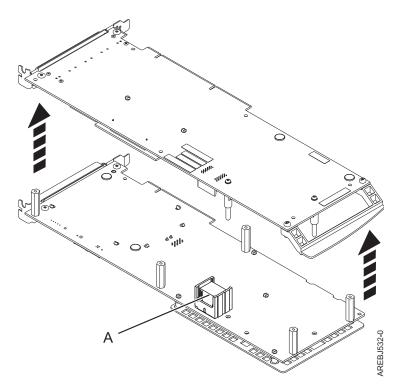
Figure 30. Location of interconnect connector on the 572F/575C card set adapter
