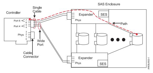
Figure 20. Example SAS subsystem
