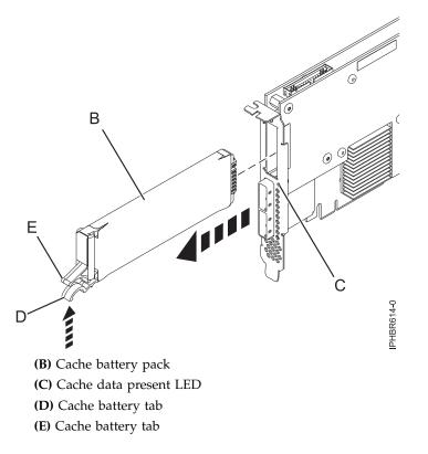
Figure 27. Replacing the 574E cache battery
