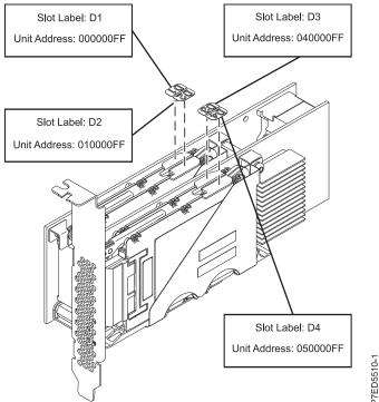
Figure 45. SAS unit addresses for CCIN 57CD PCIe SAS RAID and SSD Adapter 3 Gb x8
