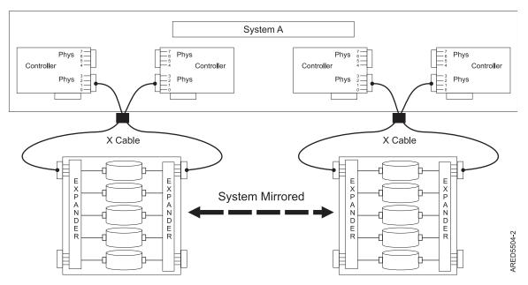
Figure 25. Dual storage IOA system mirroring configuration
