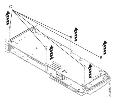
Figure 29. Location of screws on the 572F/575C card set adapter
