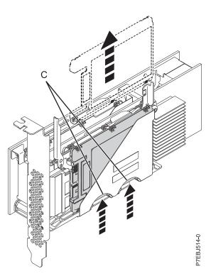
Figure 38. Pushing the SSD that is being replaced
