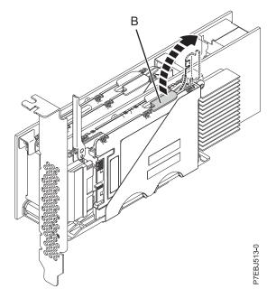
Figure 37. Lifting the device retaining latch
