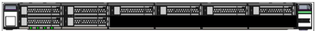
Figure 23 IBM FlashSystem 5200 NVMe drive slots supported by eight drives populated and four fillers
